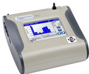
Figure 6. TSI Optical Particle Sizer (OPS) 3330 measures particulate concentrations within the primary exposure chamber of particles greater than 300 nanometers.
