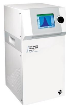
Figure 5. TSI Fast Mobility Particle Sizer (FMPS) 3091 used to monitor nanoparticle concentrations inside the chamber.
