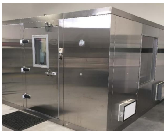
Figure 4. Stainless steel secondary aerosol containment chamber, which housed the 300-liter primary aerosol test chamber.
